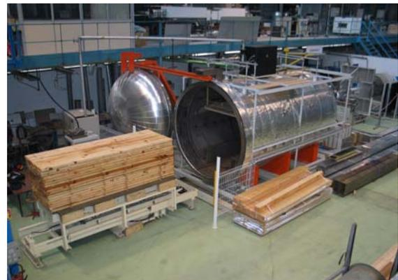
HF vapour pressure timber-drying kiln
