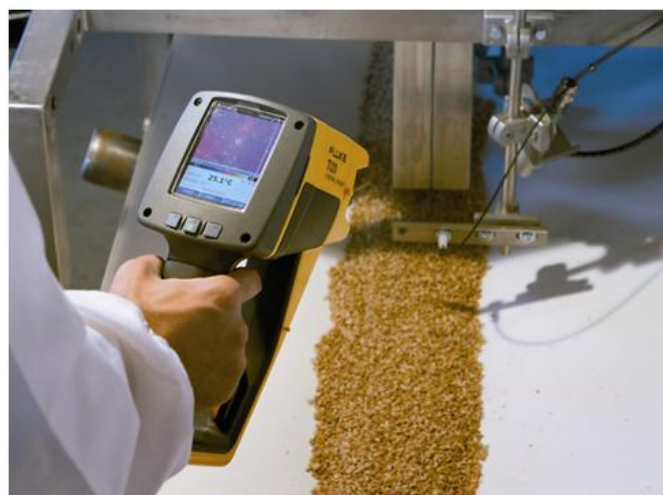
Figure 1. Legumes coming out from the microwave treatment system. Measurement of output temperatures by means of a thermocamera.
