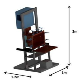
**Figure 3.** Drawing of the MEAM VP 1.2 (VP and 1.2 stand for vacuum/pressure and 1.2 kW power, respectively).
