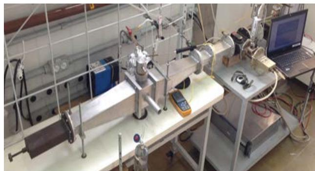
Figure 2: Microwave applicator developed for plug flow vapor phase reactor.
