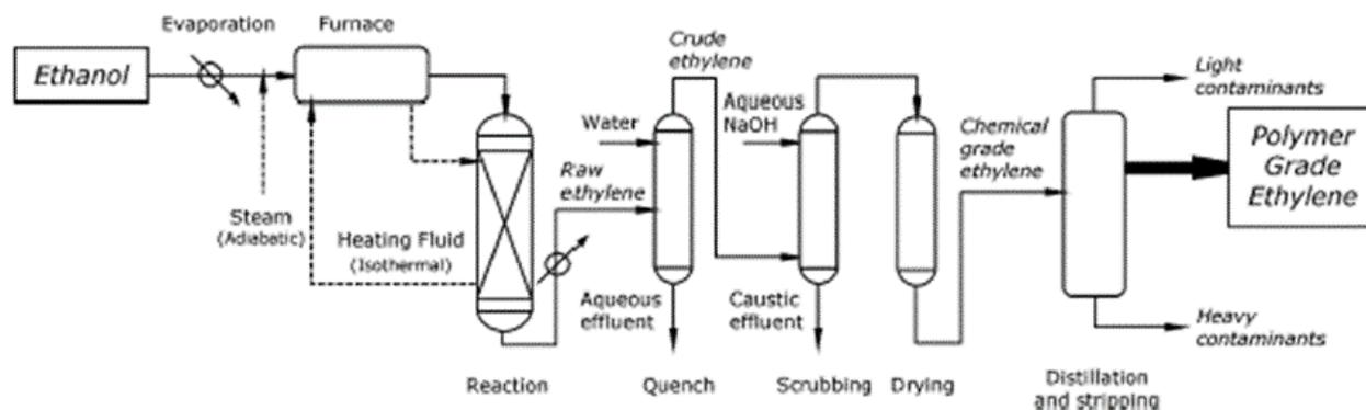
Figure 1: Typical flowsheet for ethylene via ethanol dehydration<sup>12</sup>.
