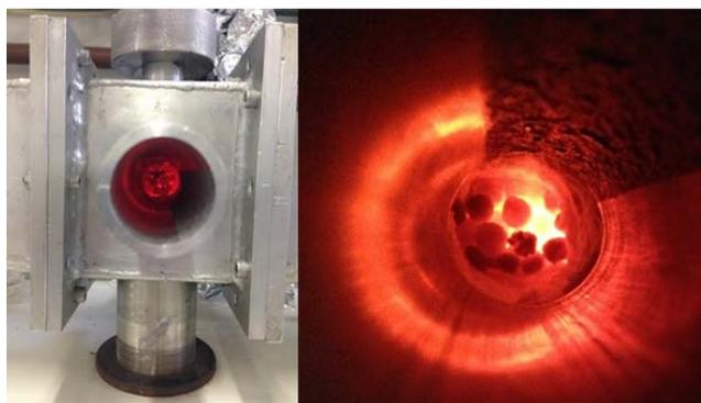
Figure 5: Details of the reaction chamber. (Left): cavity detail of parallel epipedal section, showing the heated catalytic bed. (Right): internal view of the heated catalytic bed.
