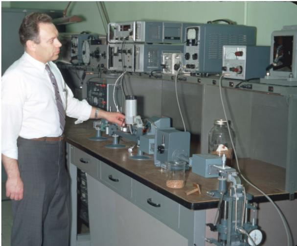
**Figure 6.** An X-Band system for 8- to 12-GHz dielectric measurements.
