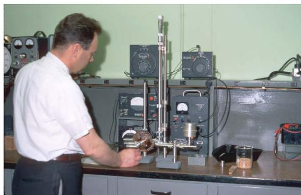
**Figure 5.** Admittance meter system for dielectric measurements in the range of 200 to 500 MHz.
