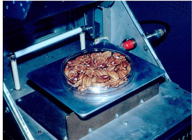
**Figure 8.** Pecan kernels on lower electrode of the dielectric heater.
