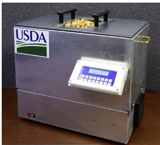
**Figure 9.** Microwave moisture meter for peanut kernel moisture measurement
