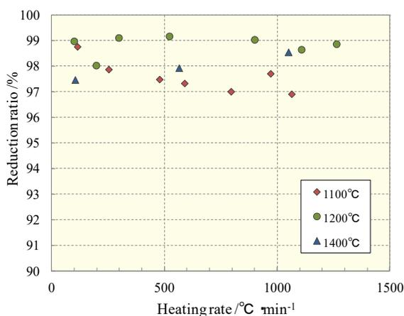
**Figure 7.** Dependence of experimental reduction ratio of  $\text{Fe}_3\text{O}_4$  on the heating rate and target temperature (1100, 1200 and 1400°C).
