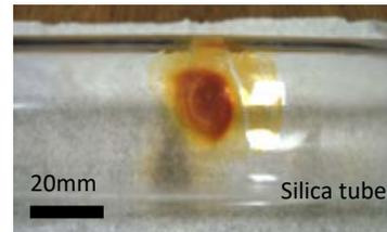
Figure 5. Photograph of phosphorous deposits on silica tube.
