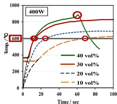
**Figure 2.** Heating curves of DPF having various metal volume fractions at 400-W power input<sup>9</sup>.
