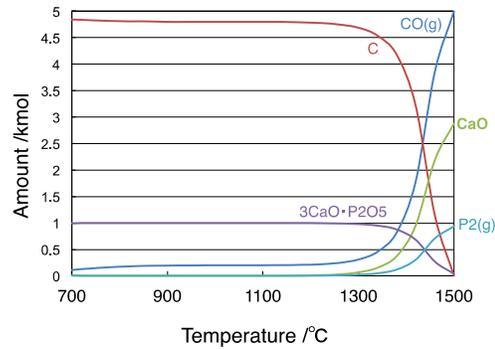
Figure 4. Calculated phase constitution at elevated temperature.
