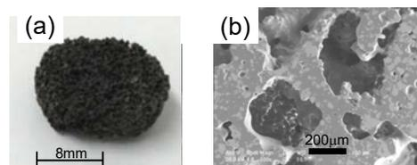
**Figure 1.** (a) The fabricated DPF, and (b) its microstructure observed with SEM. The volume fraction of stainless steel particles is 30%.
