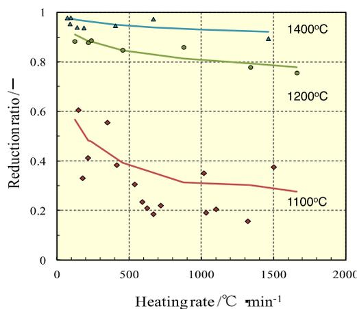
**Figure 6.** Dependence of experimental reduction ratio of TCP on heating rate for three target temperatures (1100, 1200 and 1400°C); the calculated data are shown by lines.
