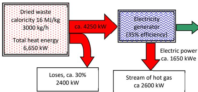
Figure 8. Energy balance for the system of microwave gasification of waste with calorificity of ~16 MJ/kg.
