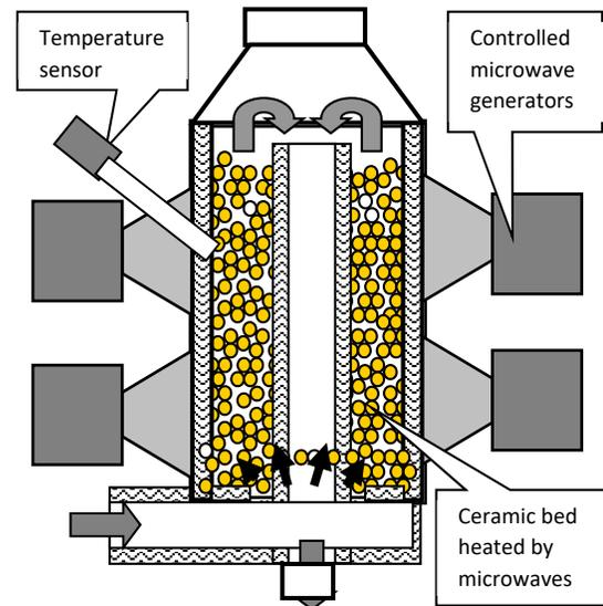
Figure 3. MOS construction scheme.
