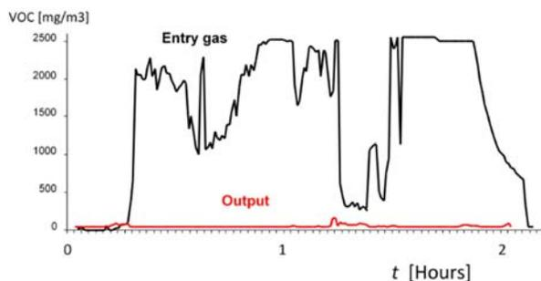
**Figure 4.** Measurements of volatile organic compounds (VOC) before and after MOS reactor.
