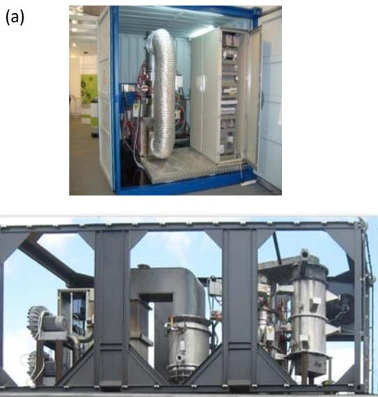
**Figure 5.** MOS reactors installed in 20-feet containers, with capacities of 600 m<sup>3</sup>/h (a) and 4500 m<sup>3</sup>/h (b).
