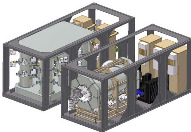
**Figure 10.** System for asbestos treatment installed within two standard containers.
