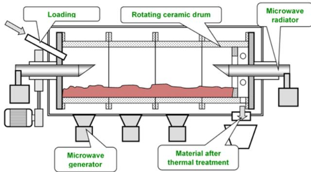
Figure 1. A schematic of the HR reactor.
