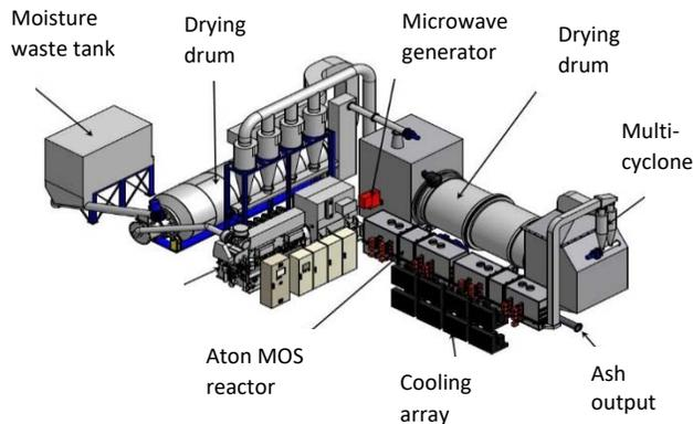
Figure 7. A system with HR 5000 reactor.
