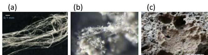
**Figure 9.** (a) Chrysotile asbestos, (b) asbestos fibers in shredded Eternit, and (c) ATONIT, a product of Eternit processing in the microwave reactor by the MTT technology.
