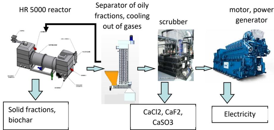
Figure 6. Installation for utilization of municipal waste with electricity production.
