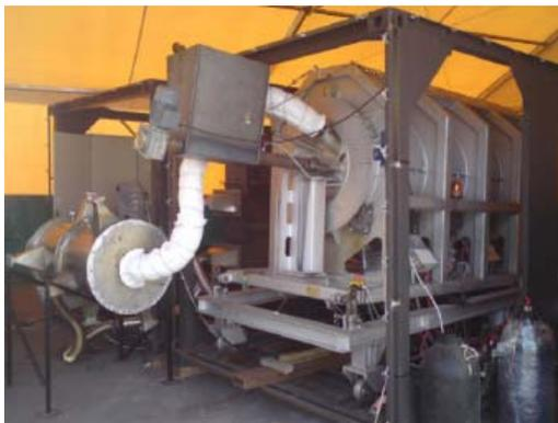
Figure 2. The HR-200 reactor installed inside a standard 20-foot container.
