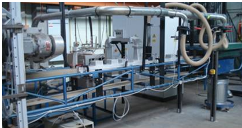
Microwave system for remediation of oil contaminated drill cuttings
