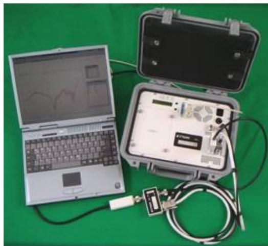
Fig. 1. InSite multipurpose portable “cold measurement” system.
