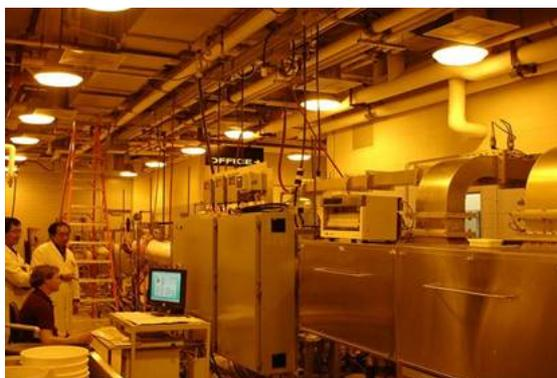
**Fig. 2.** WSU engineers (Zhongwei Tang, Frank Younce and Frank Younce) with the third generation 915 MHz pilot scale MATS system (24 m in total length). It consists of four single-mode cavities and pressurized chamber to allow processing of 50 meals in a semi-batch mode.
