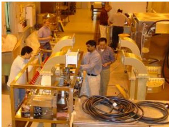
**Fig. 1.** Engineers and students assembling the 2nd generation pilot-scale 915 MHz MATS system in 2002. It had two heating cavities, and could process four food packages in a batch mode.
