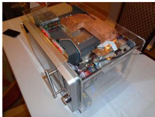
Figure 3. Huber+Suhner: domestic microwave oven with a solid-state amplifier as power source
