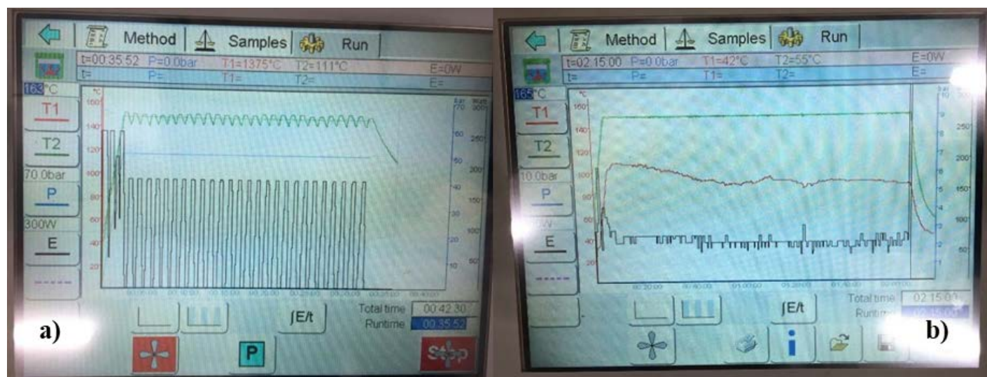
Figure 3. a) typical temperature (green line)/power (black line) profile when using vessel setup: intermittent power delivery leads to up to 10 °C temperature oscillation around the set value. b) typical temperature (green line)/power (black line) profile when using flask setup: a homogeneous power delivery leads to a stable temperature. Note the red line which is the temperature measured by the thermocouple.
